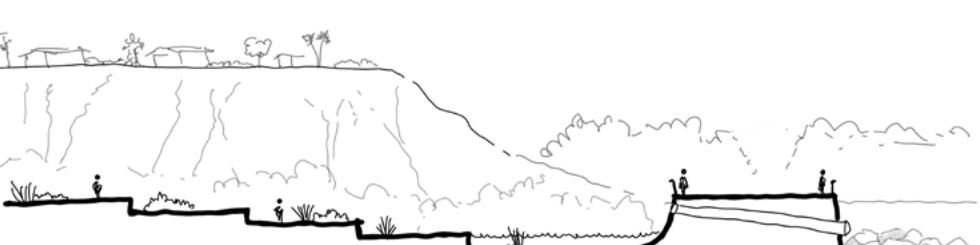
B: TERRACED ARROYO DETENTION BASIN
