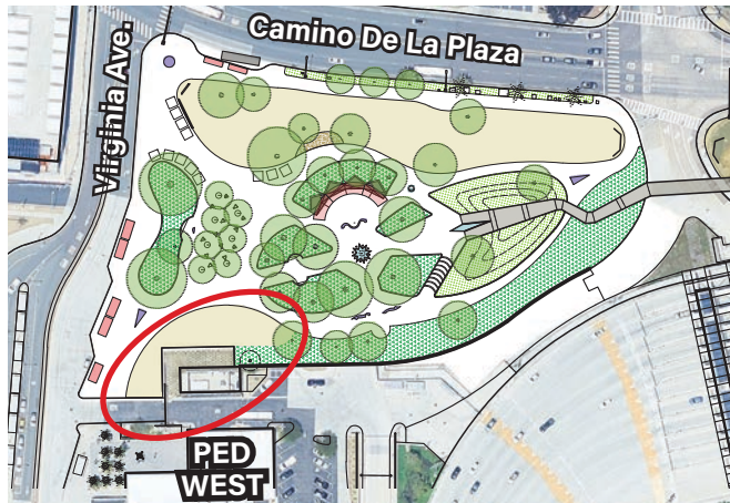
Bioretention Basin Added
