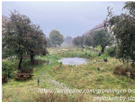
Example: Multi-use infiltration basin-wet weather
